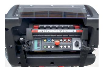
Platforms equipped with lithium-ion have integrated diagnostic systems that make it possible for the operator to identify any anomalies, and to monitor the battery pack's primary operational parameters directly from the remote display. First an icon and an acoustic signal, then the progressive slowing down of the machine's movements alert the operator when the battery is about to run out. In case of malfunction, the operator is notified with specific error codes shown directly on the display.
