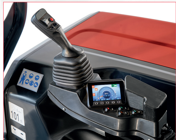
All the fundamental machine controls are on the joystick: hydraulic pump control, bucket control, accelerator, horn and speed.
